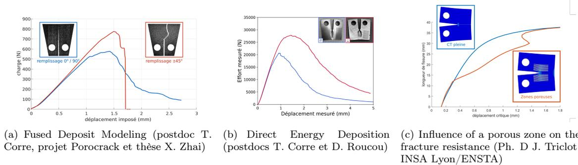
Figure 1: Influence of the microstructure on crack propagation
